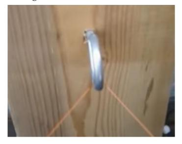
You're going to "walk the line" back and forth a total of 24 times (to make 23 AWG wire).
