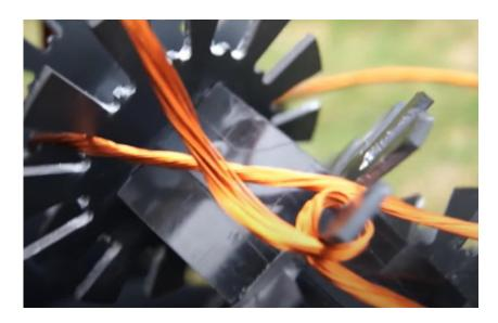
Note: Make sure that you begin the next loop behind the Input 1 wire. You're going to want Input A to point out of the coil so the ends are readily available.
