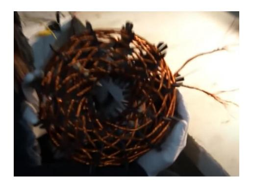
The remainder of the spooled wire should be about the same length as the 'Input 1' wire. The remainder will help form your 'Input 2' wire.
