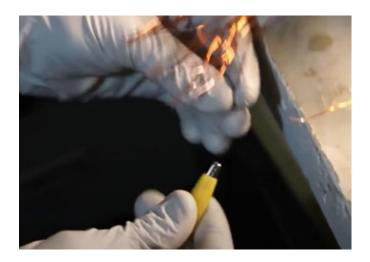
Now take the "negative" banana connector and touch it to any of the exposed wires on the Input 2 wire.
