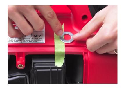
**Step 3:** Mark your hole, and start drilling with the pilot bit before increasing it 9/16" using your step bit.
