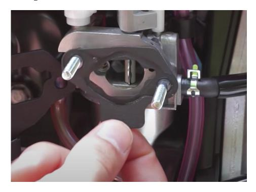
**Step 7:** Replace the air filter assembly with a spacer included in your kit.
