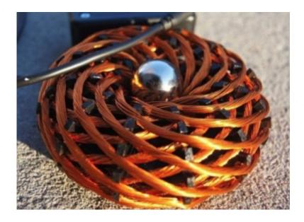
You see, as current travels **counter-clockwise** through the inner winding, the same current travels clockwise through the outer winding...
